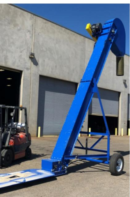
**Cambelt's Portable Car Unloader Scorpion 1210PCU** is among our most durable and versatile unloaders. It features one of the smallest footprints in the industry while offering load rates up to 1,350 cubic feet per hour.
