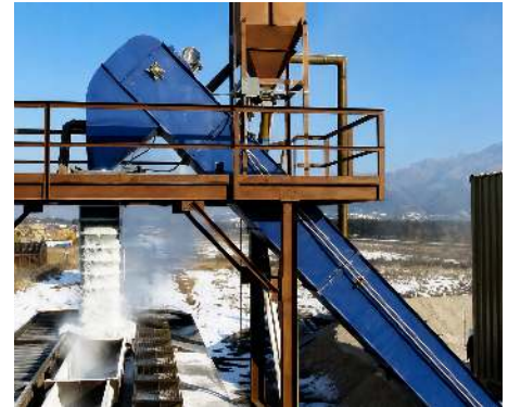
SODA ASH: UNLOADING 80,000 LBS. IN 20 MINUTES (120 TPH)
