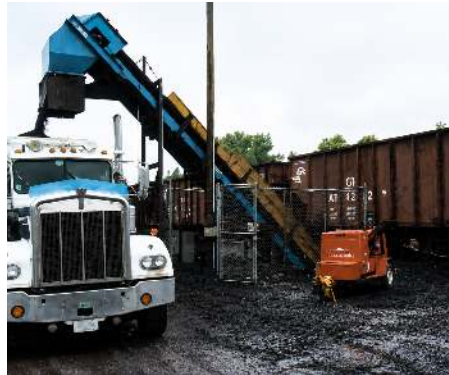
COAL: LOADING 24 TONS IN 4 MINUTES (360 TPH)
