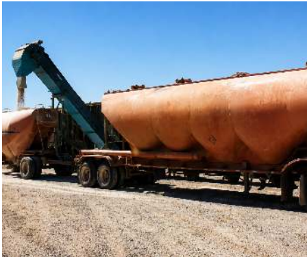
PEBBLE LIME: UNLOADING AT 150 TPH
