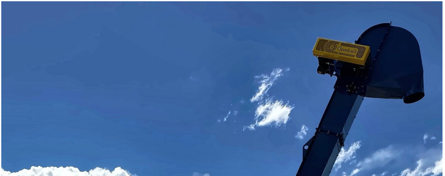
THE DISCHARGE HEAD, 15'-4" UP A 60° INCLINE.
