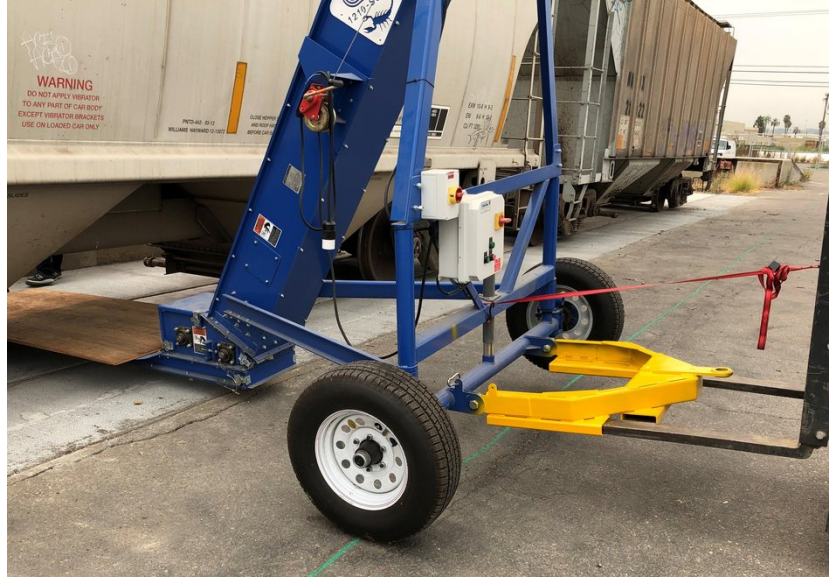
TOWED IN BY FORKLIFT, INLET UNDER THE HOPPER CAR.
