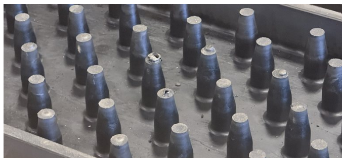
MONOLITHIC SBR CAMBELT: NUBS AND SIDEWALL MOLDED AS ONE.
