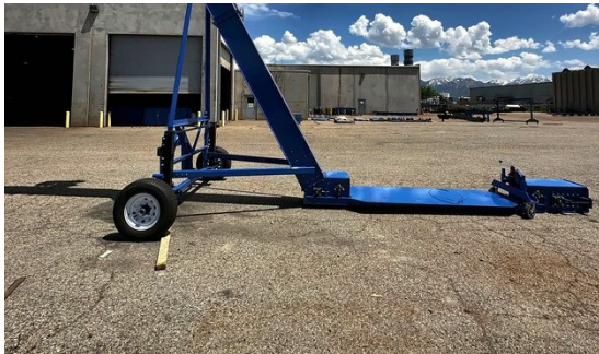
LOW-PROFILE INLET, TOW END AND LIFT JACKS.
