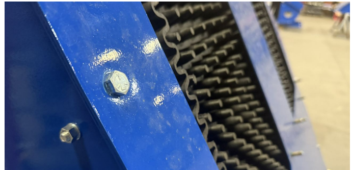
THE BELT RUNNING INSIDE THE ENCLOSED CONVEYOR.
